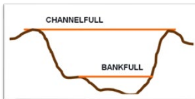
Figure 2. Stream cross-section illustrating channelfull versus bankfull in an incised channel.
